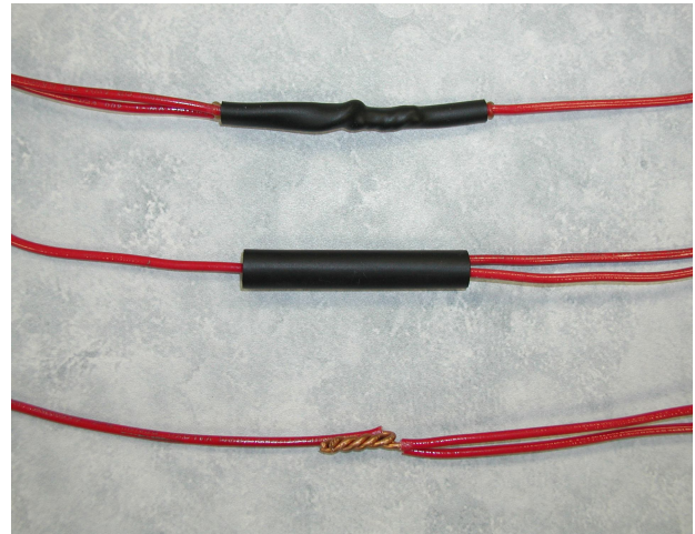
Meltable inner liner for encapsulating
